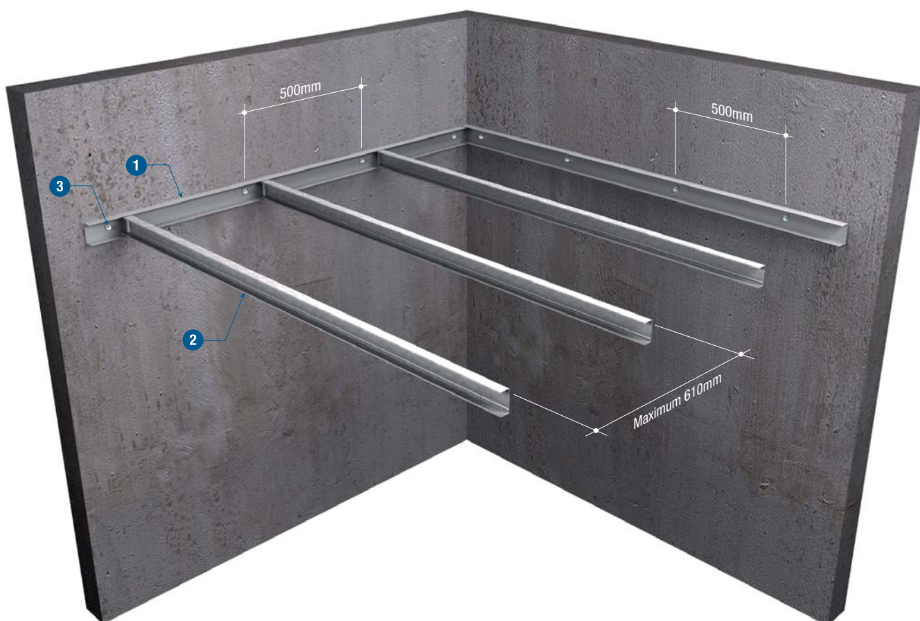
Fixing of primary and secondary profiles
